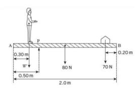
A student is being weighed. The student, of weight (W), stands 0.30m from end A of a uniform plank AB. The plank has a weight of 80N and length 2.0m. A pivot P supports the plank and is 0.50m from end A. A weight of 70N is moved to balance the weight of the student. The plank is in equilibrium in the diagram.
